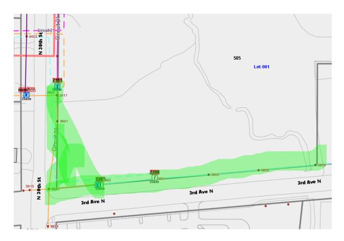
**Location 2: North of Danforth Rd near RR tracks** – Three phase line north of Danforth Rd and east of the RR Tracks, beginning at Danforth Rd north to Pole #4339, including the tap from Pole #4336 to Pole #4334 and from Pole #4332 to Pole #4331. Remove all trees, limbs, saplings, and brush ground to sky **within 20 feet of the centerline of the power line**, plus the standard aerial 10-foot line clearance as defined in the Technical Specifications. Area highlighted in green.
