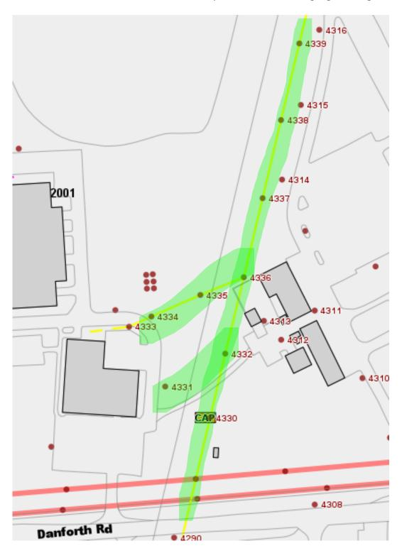
**Location 3: College Avenue** – Three phase line south of College Avenue from Pole #4364 near the intersection of N 30<sup>th</sup> St heading east to Pole #4369. Remove all trees, limbs, saplings, and brush ground to sky within 15 feet of the centerline of the power line, plus the standard aerial 10-foot line clearance as defined in the Technical Specifications. Area highlighted in green.
